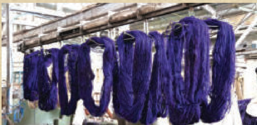
Overhead Chain -Link System 4m Long For Drying of Dyed Jute Hanks by Sun & Wind
