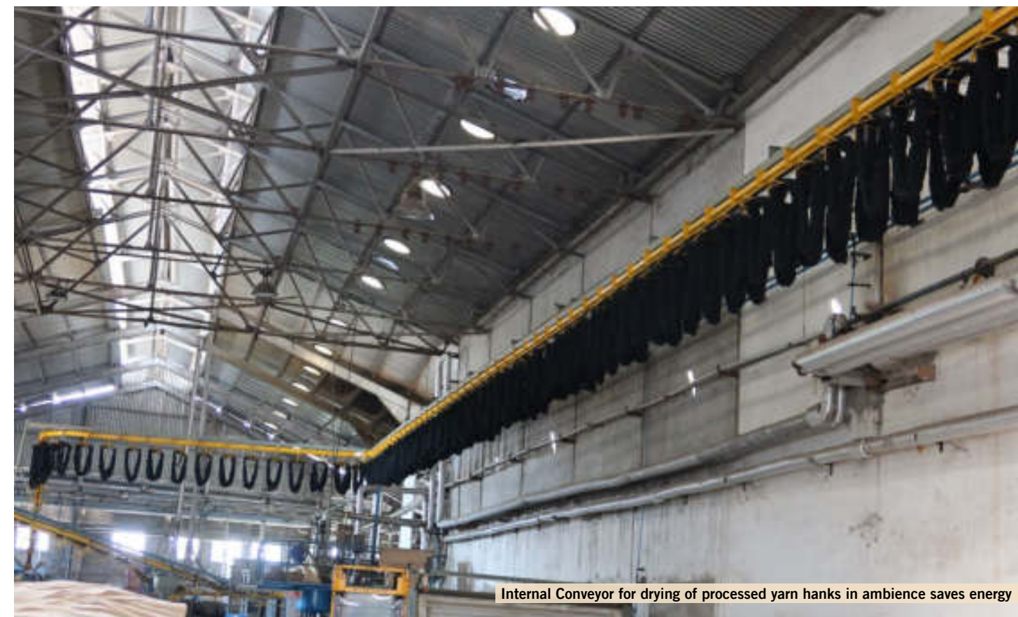
Open Air Conveyor for drying of processed yarn hanks saves energy
